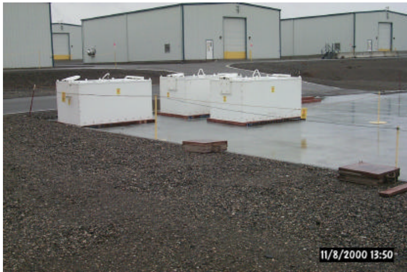
Fig. 1. Failed RH-TRU Equipment and Debris Stored in Shielded Boxes
