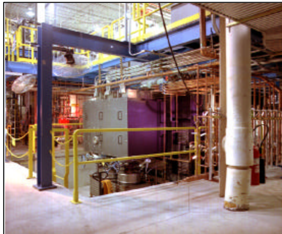
Fig. 2. Simulated low-activity waste vitrification demonstration in one-third-scale pilot plant melter.
