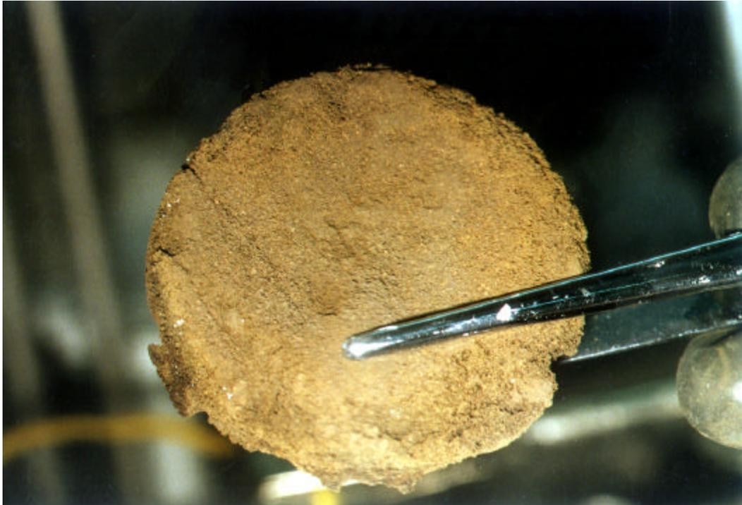
Fig. 4: The crumbly disposal product of silica reacted with sodium, containing elemental Si,  $\text{Na}_2\text{SiO}_3$ , and excess  $\text{SiO}_2$ .
