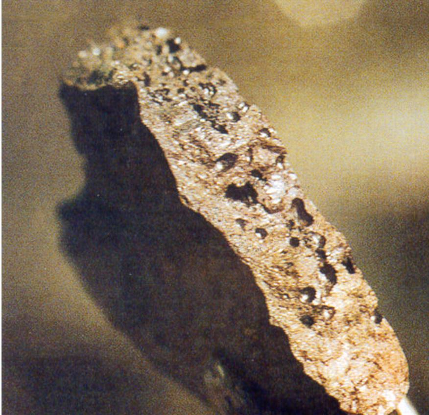
Fig. 3: Shows the final product, "hockey puck" formed by magnetite in a 3:1 stoichiometric mixture with 35g sodium, cracked to show the interior of metallic Fe,  $\text{Na}_2\text{FeO}_3$ ,  $\text{Na}_2\text{O}$ , and excess  $\text{Fe}_3\text{O}_4$ .
