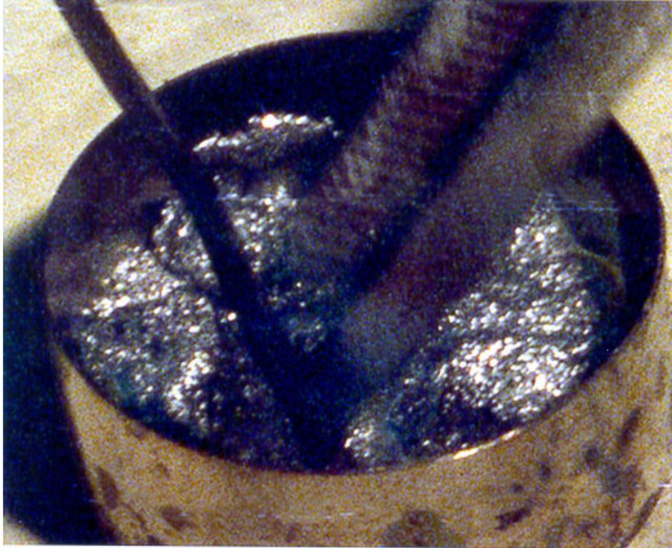
Fig. 2: Shows 1:1 stoichiometric ratio mixture of sodium with feed material at mixing temperature, slowing ramping to initiation temperature.
