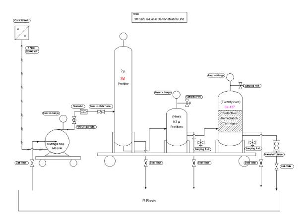
Fig. 1. 3M SRS R-Basin Demonstration Unit Schematic
