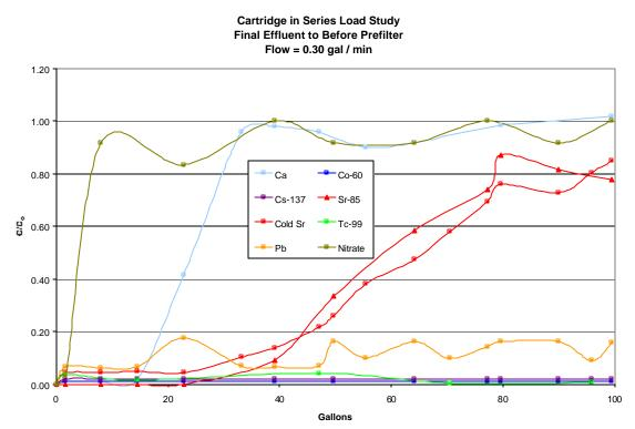
Fig. 4. Cartridge in Series Load Study Results
