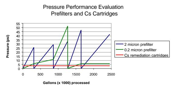
Fig. 3. 3M SRS R-Basin Pressure Performance
