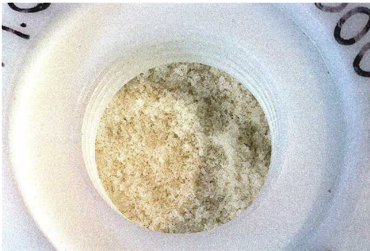
Fig. 1: Solidified Oil in Burial Liner – Top View
