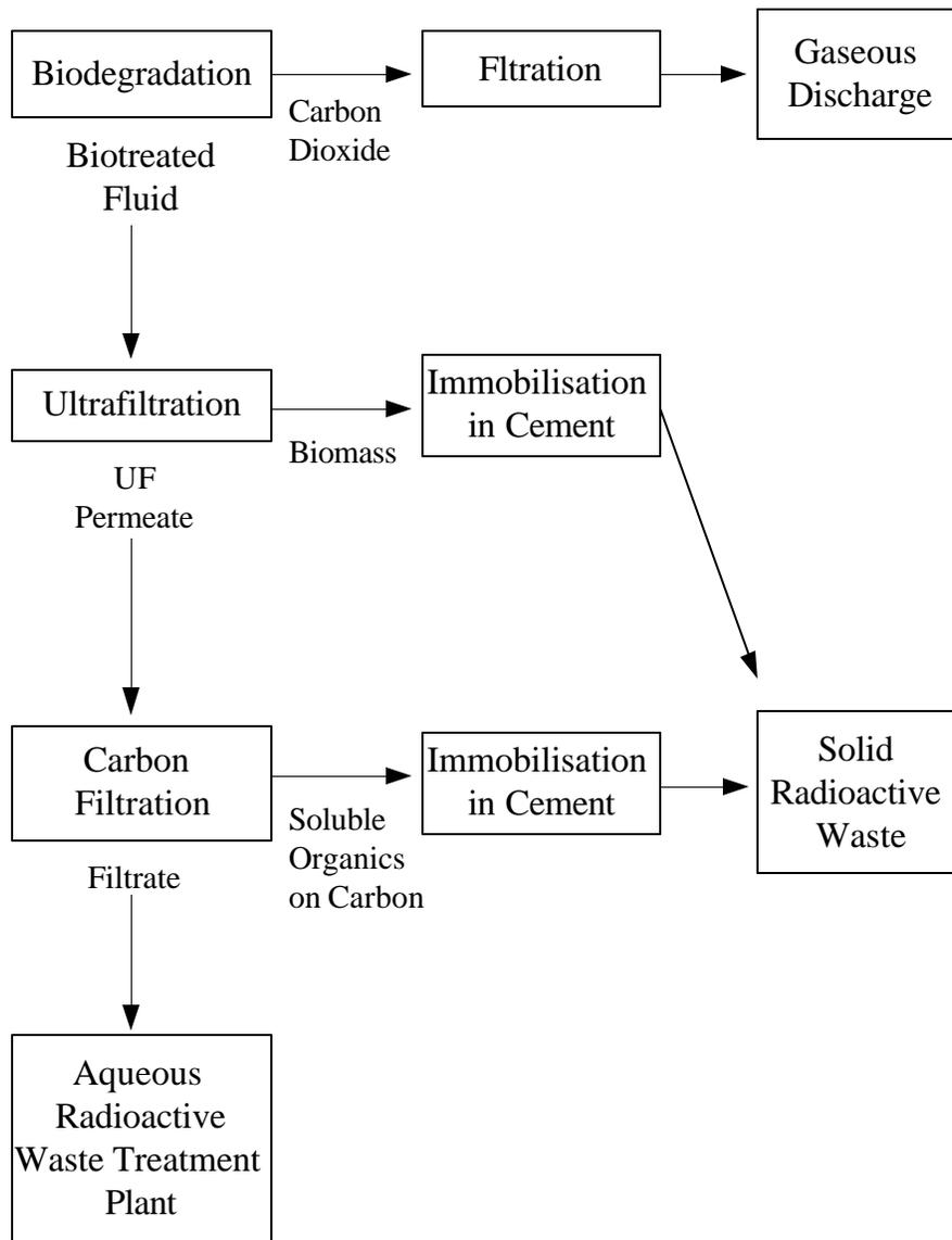
Fig. 2. Proposed Treatment Process for Waste Radioactive Cutting Fluid
