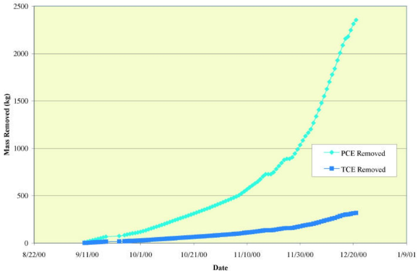
Fig. 4. Plot of contaminant mass removal from September 10 through December 21 for the DUS project at SRS.
