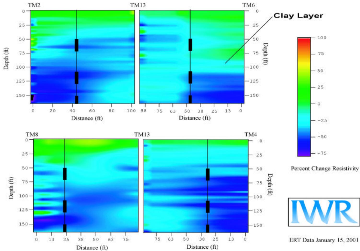
Fig. 3. ERT percent change in resistivity between data collected 1/15/01 and background collected 8/24/00.
