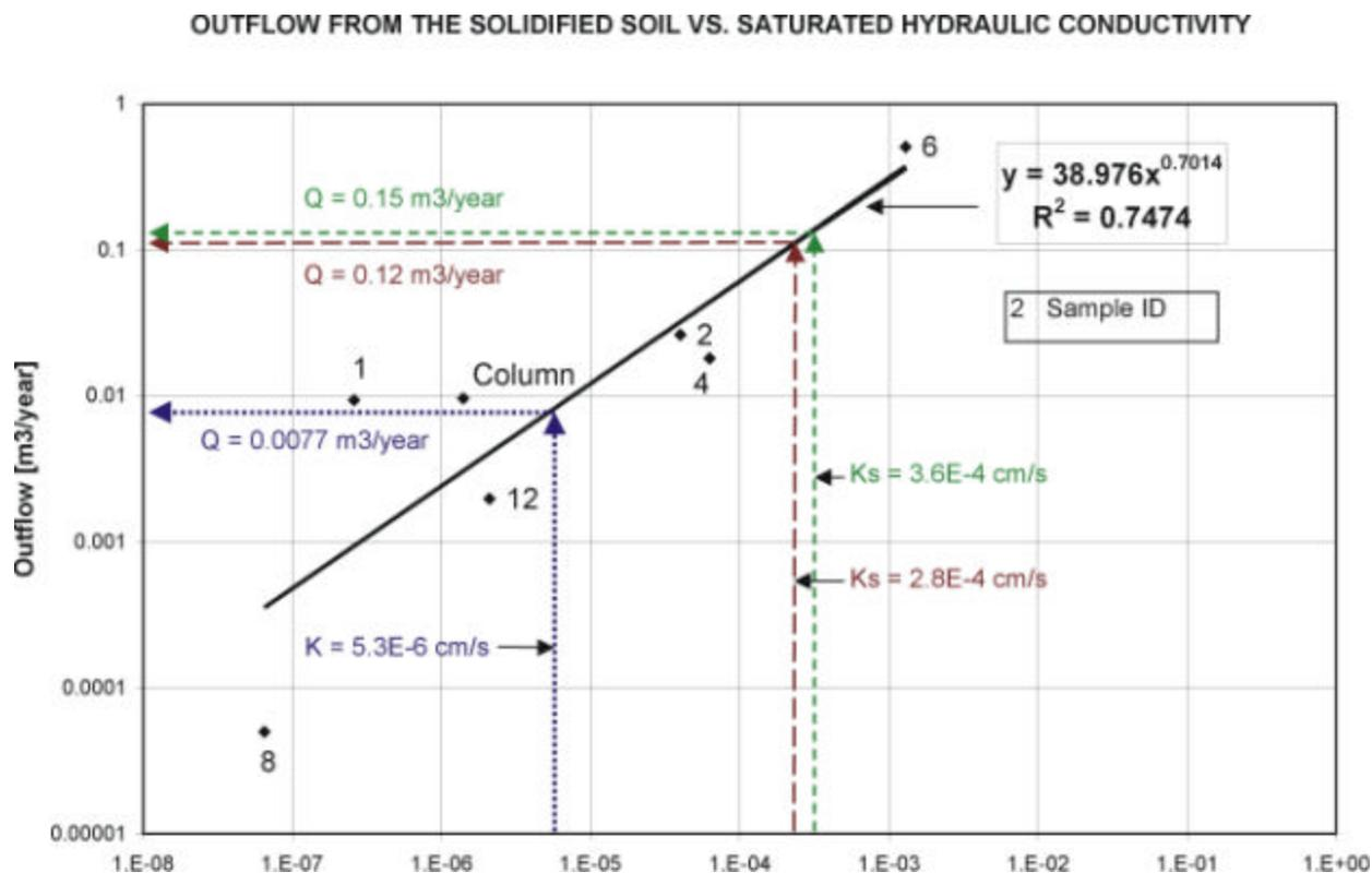
Fig. 4. Plot of Saturated Hydraulic Conductivity (cm/sec) vs. Outflow (m<sup>3</sup>/yr).
