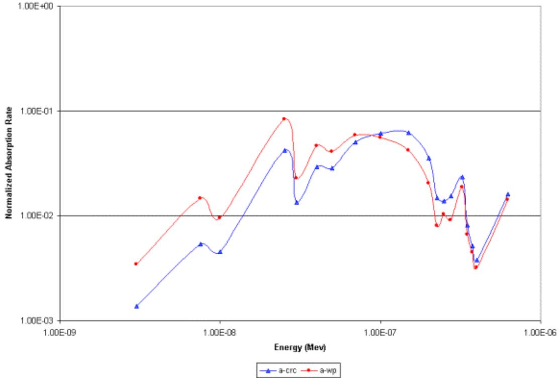
Fig. 1. Absorption Reaction Rate in the Fuel Region of the WP and CRC
