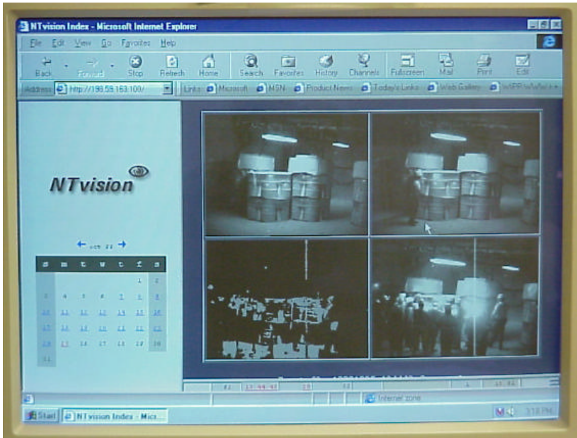
Figure 3. Output video screen of the NTVision surveillance system detecting intrusion into the underground WIPP demonstration area.
