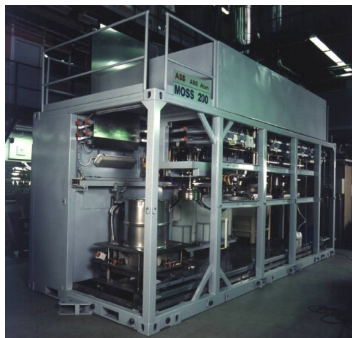
Figure 2: Photo of the MOSS 200 unit delivered to the Borssele Nuclear Power Plant
