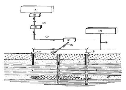
1 - TREATMENT PLANT, 2 - TRANSFER PUMPING STATION, 3 - LOW-PRESSURE PIPELINES, 4 -HOLDING TANK BUILDING AND INJECTION PUMPING STATION, 5 - HIGH–PRESSURE PIPELINE, 6 -INJECTION WELL, 7 - OBSERVATION MONITORING WELL, 8 - COLLECTION OF MONITORING DATA, 9 - ADMINISTRATIVE AND ENGINEERING BUILDING, 10 - RESERVOIR FORMATION, 11 - WASTES IN RESERVOIR.
