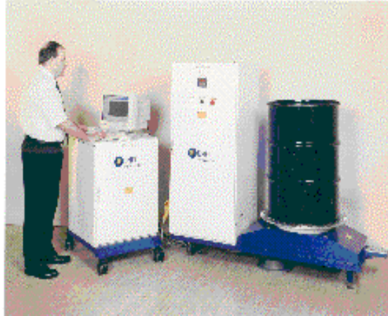
Figure 1 BNFL Instruments DrumScan ® : LRGS system in 200liter drum monitoring configuration and incorporating a separate workstation which can be located remote from the measurement unit to reduce operator dose uptake.
