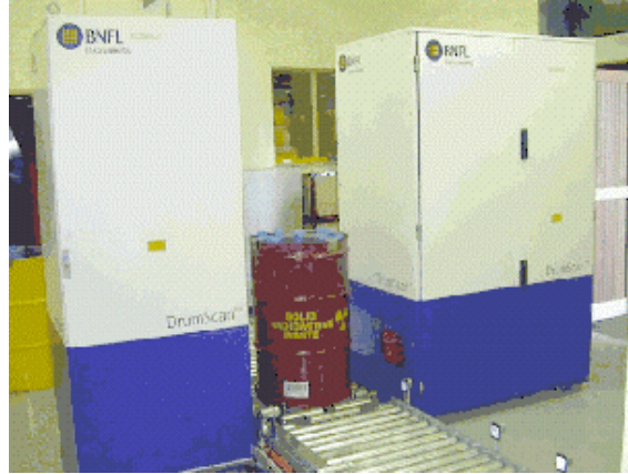
Figure 2 BNFL Instruments DrumScan ® : HRGS in 200liter drum monitoring configuration
