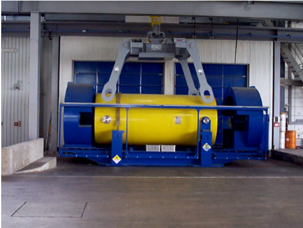
Fig. 2: MOSAIK 80 T transport cask filled with fuel element boxes in front of the transport cask lock
