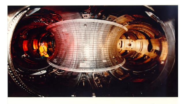
Figure 1 - Internal TFTR vessel (prior to tritium operations)
