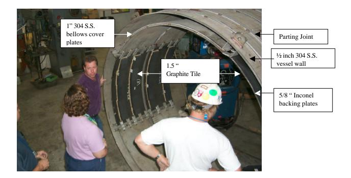
Figure 2 Vacuum vessel surrogate prior to filling
