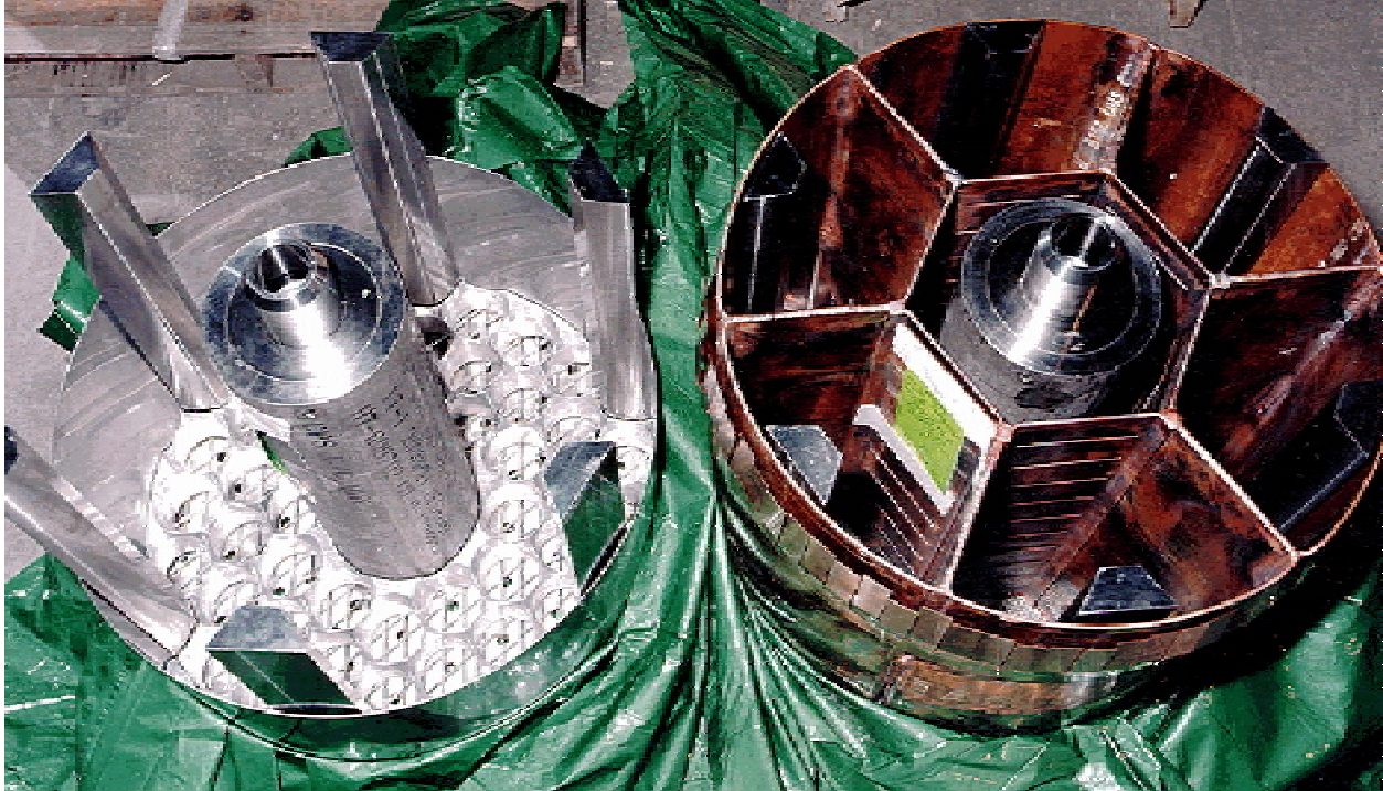
Figure 3. Mark 1A prototype fuel (L) and scrap baskets. Note the copper segment dividers in the scrap basket, and the large diameter stainless steel center post in both baskets.
