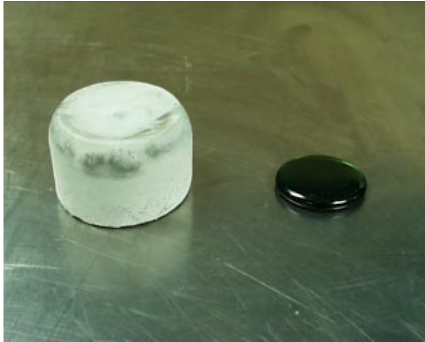
Figure 2. Final Volumes for Cementation and Vitrification of Evaporator Bottoms
