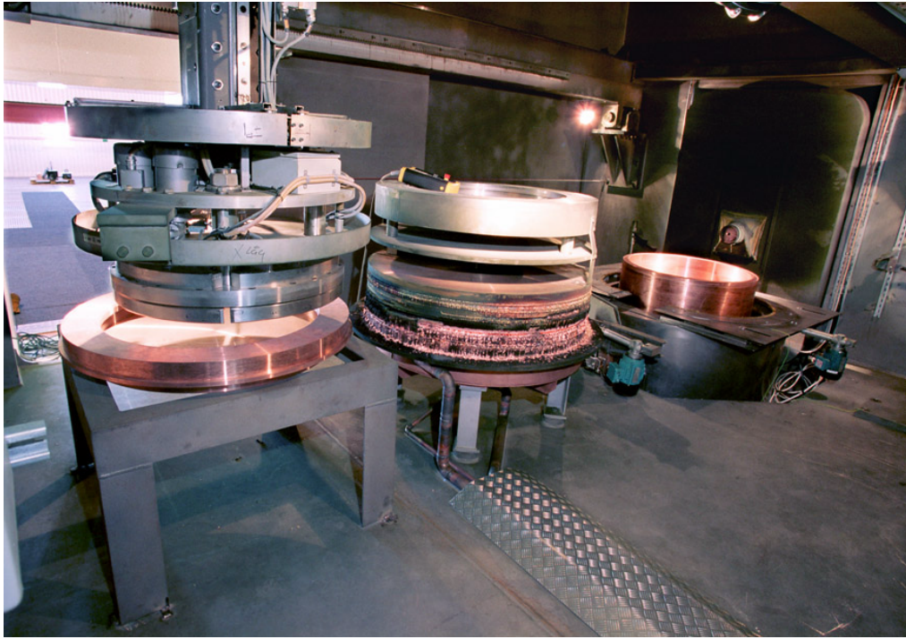
Figure 4. Vacuum chamber for electron beam welding of the copper lid
