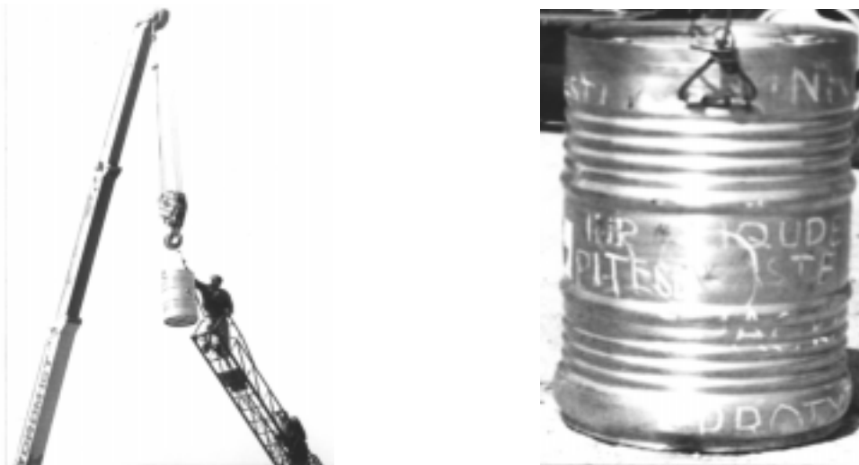
Fig. 4 The 9m free drop test for CDF-1 package designated to liquid wastes (before and after)
