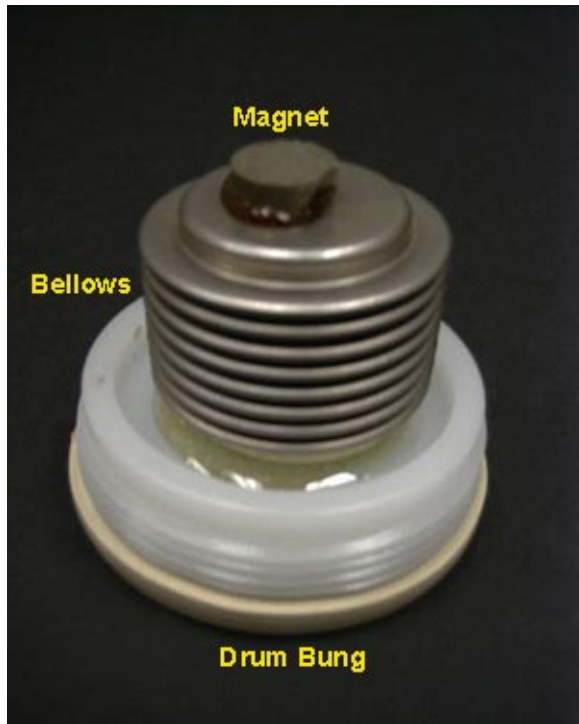
Figure 1. The pressure sensor consists of a magnet and bellows attached to the inside of a drum bung or drum lid.
