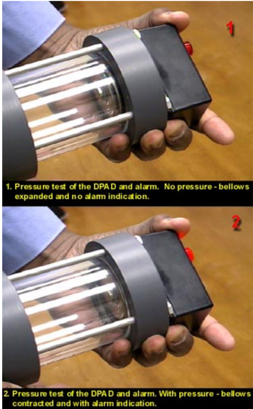
Figure 2. Tests of bellows with attached magnet and pressure alarm.
