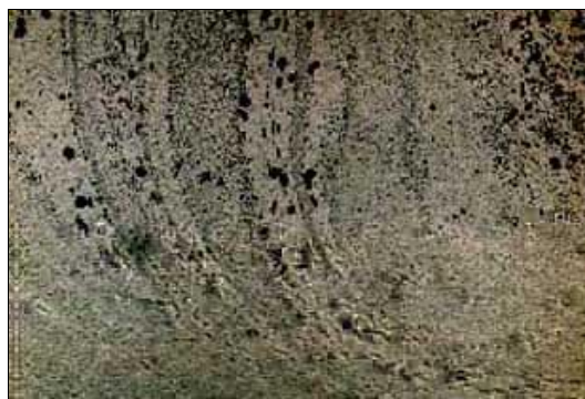
Fig. 1. Micrograph of thin section of the sample prepared by the CCIM method (optical microscopy; transmitted light; parallel nicols; magnification, 15 x , grey regions – glass, small black crystals – inclusions of zirconium phase)
