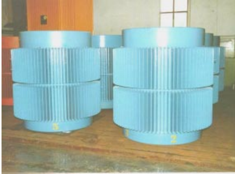
Figure 2 Illustration of CASTOR cask showing general appearance and cast in cooling fins.
