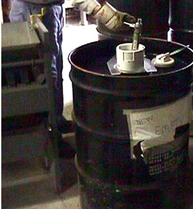
Fig. 1. Loading of well-logging sources into Type A shipping container.
