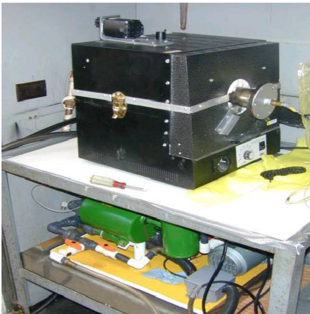
Fig 1. Bench-scale indirectly heated high vacuum rotary thermal desorption and destruction process unit
