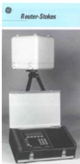
Figure 1. The RSS-112 PIC Portable Environmental Radiation Monitor Setup
