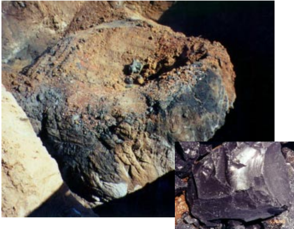
Figure 3. Vitrified Monolith Created During the Cold Demonstration
