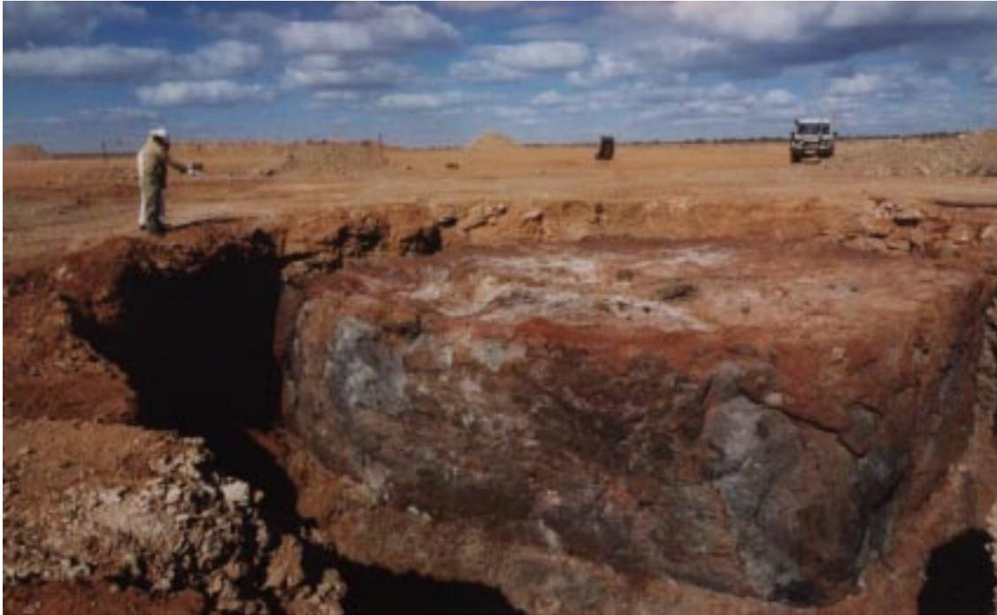
Figure 3. 500 tonne vitrified monolith resulting from the treatment of Taranaki Pit 19A.
