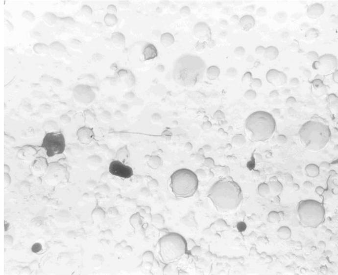
Figure 3. Phase separation of the vitreous phase in the glassy slag GS-1. Magnification, x50000.
