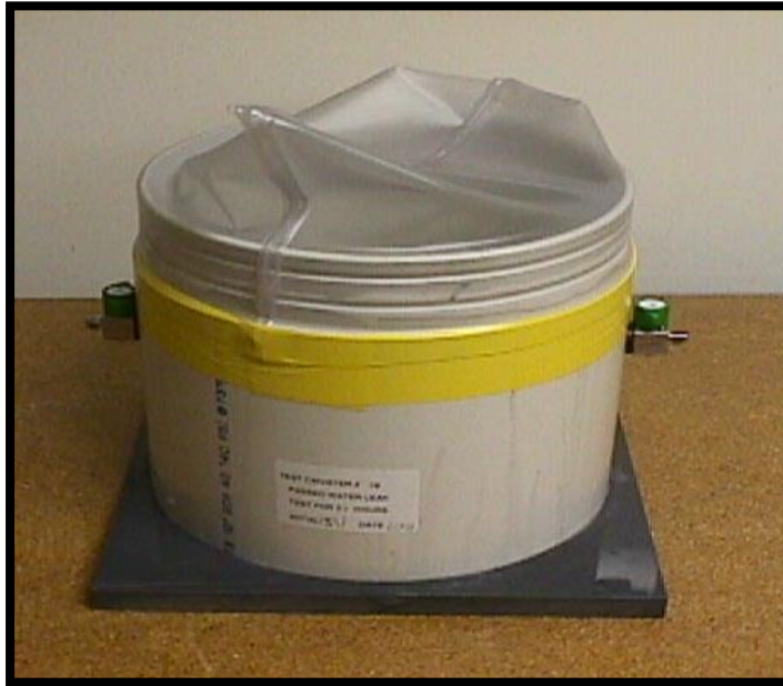
Figure-1 Polyvinyl Chloride Bag (PVC) bag-out-bag with heat-sealed end attached to test vessel
