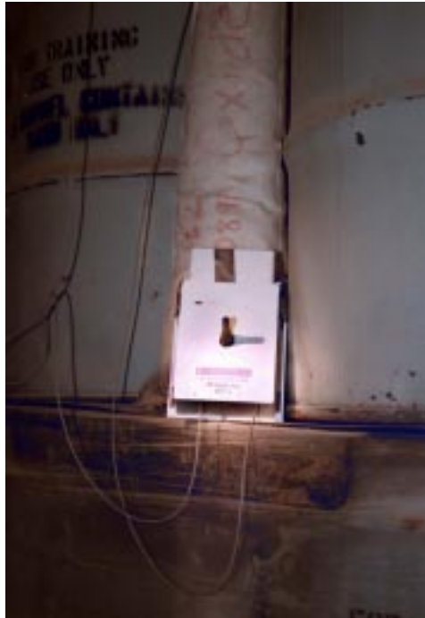
Figure 3 T-1 Electronic Sensor Platform with Fiber Optic Seal
