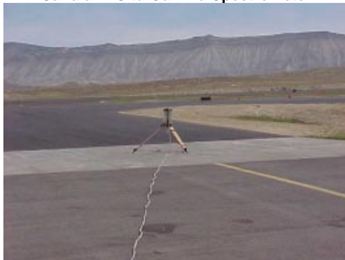
Figure 5-3 Sandia In-Situ Gamma Spectrometer
