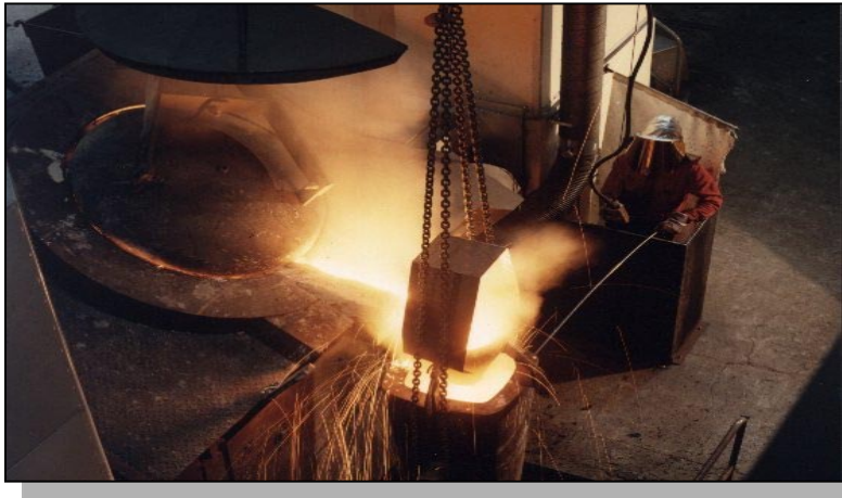
Figure 1 Pouring the melt into a mould
