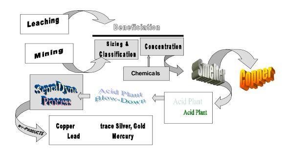
Figure 1. Copper Mining and By-Product Recovery Operations
