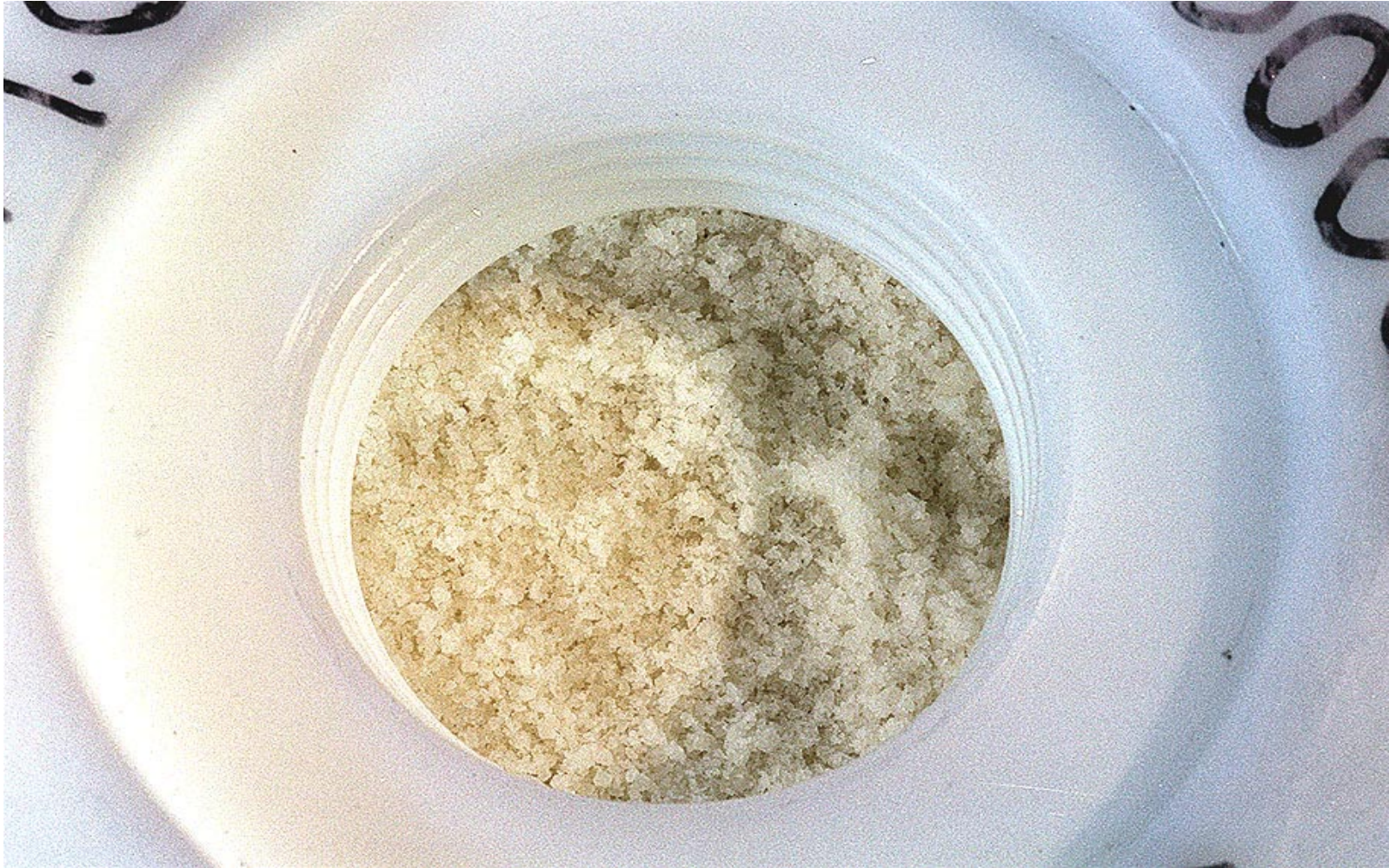
Figure 3: Solidified Oil in Burial Liner – Top view
