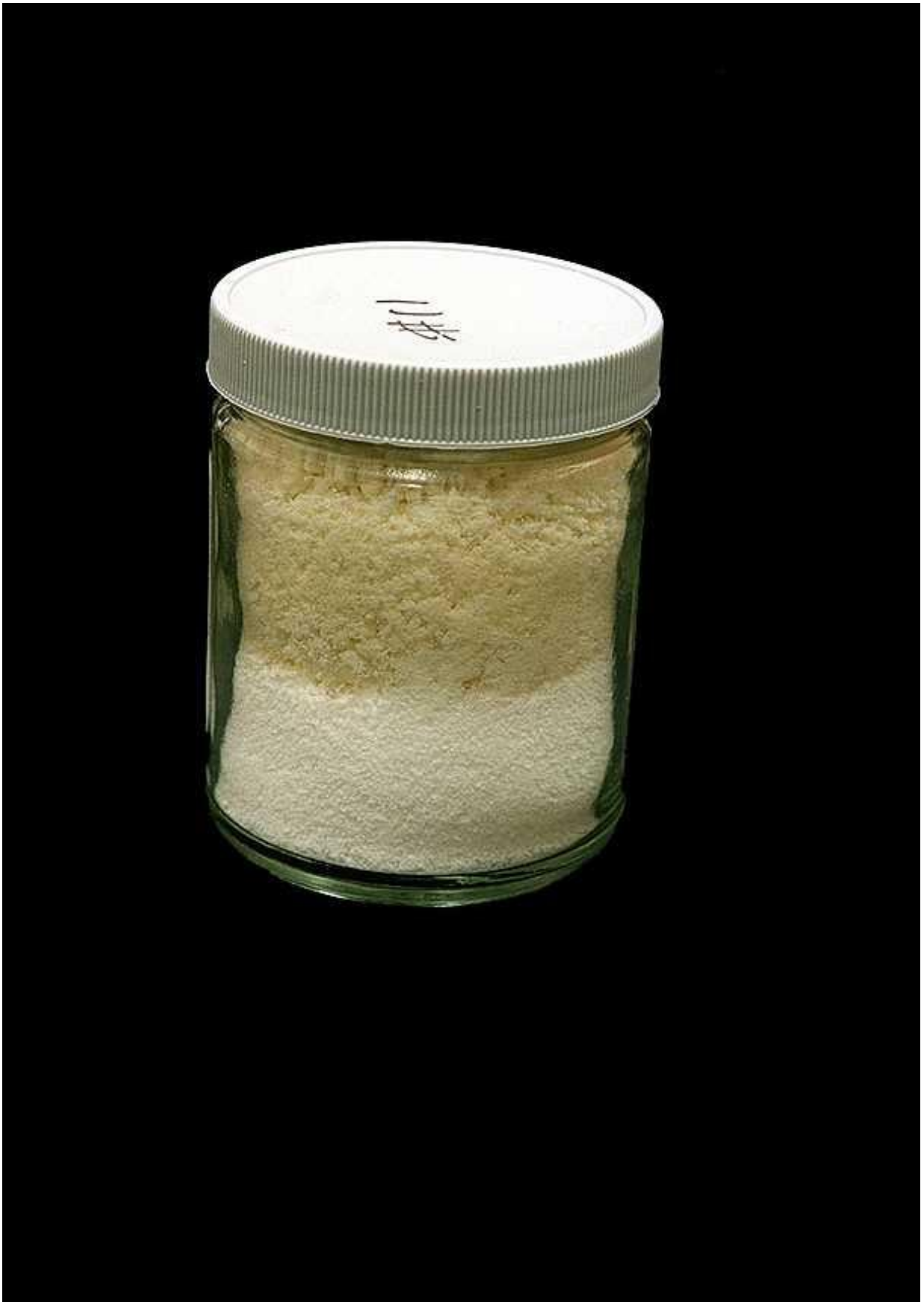
Figure 2: Solidified RCRA Oil Sample with Stratification
