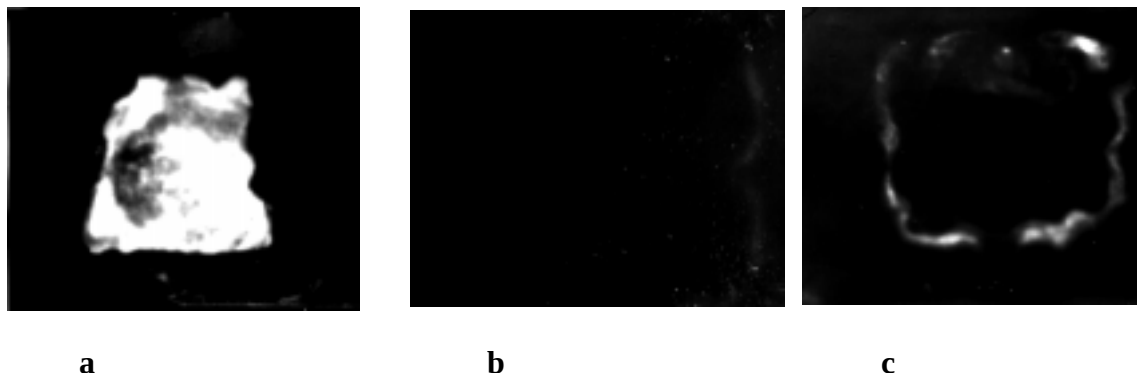
Figure 3. Autoradiographical images of stainless steel surface contaminated by Cs-137 before (a) and after (b) decontamination and autoradiogram slag surface which contacted with contaminated metal(c).
