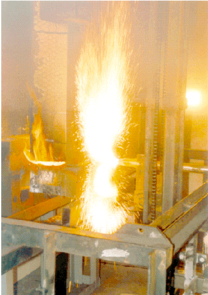
Figure 3) Remote flame cutting with iron powder injection - successful at reliably cutting through a 300m composite of steel and insulation.
