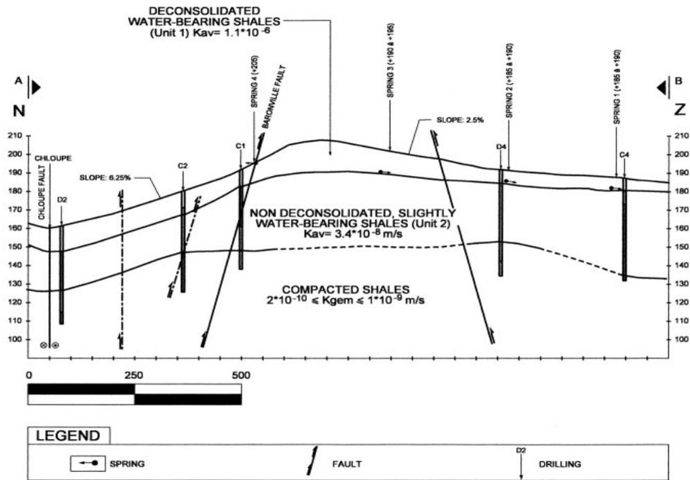
**Figure 3 : Cross section through the site**
