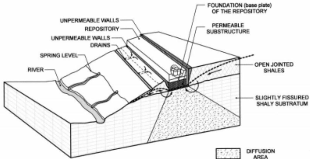
**Figure 1 : Cross section through the repository and underlying shale formations**
