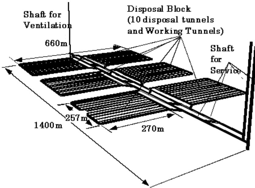
Fig. 1. Bird's-eye view of designed tunnel type repository ( Case 1 )
