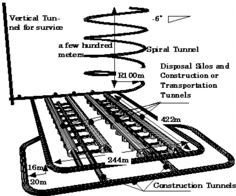
Fig. 2. Bird's-eye view of designed Underground silo type repository ( Case 3 )
