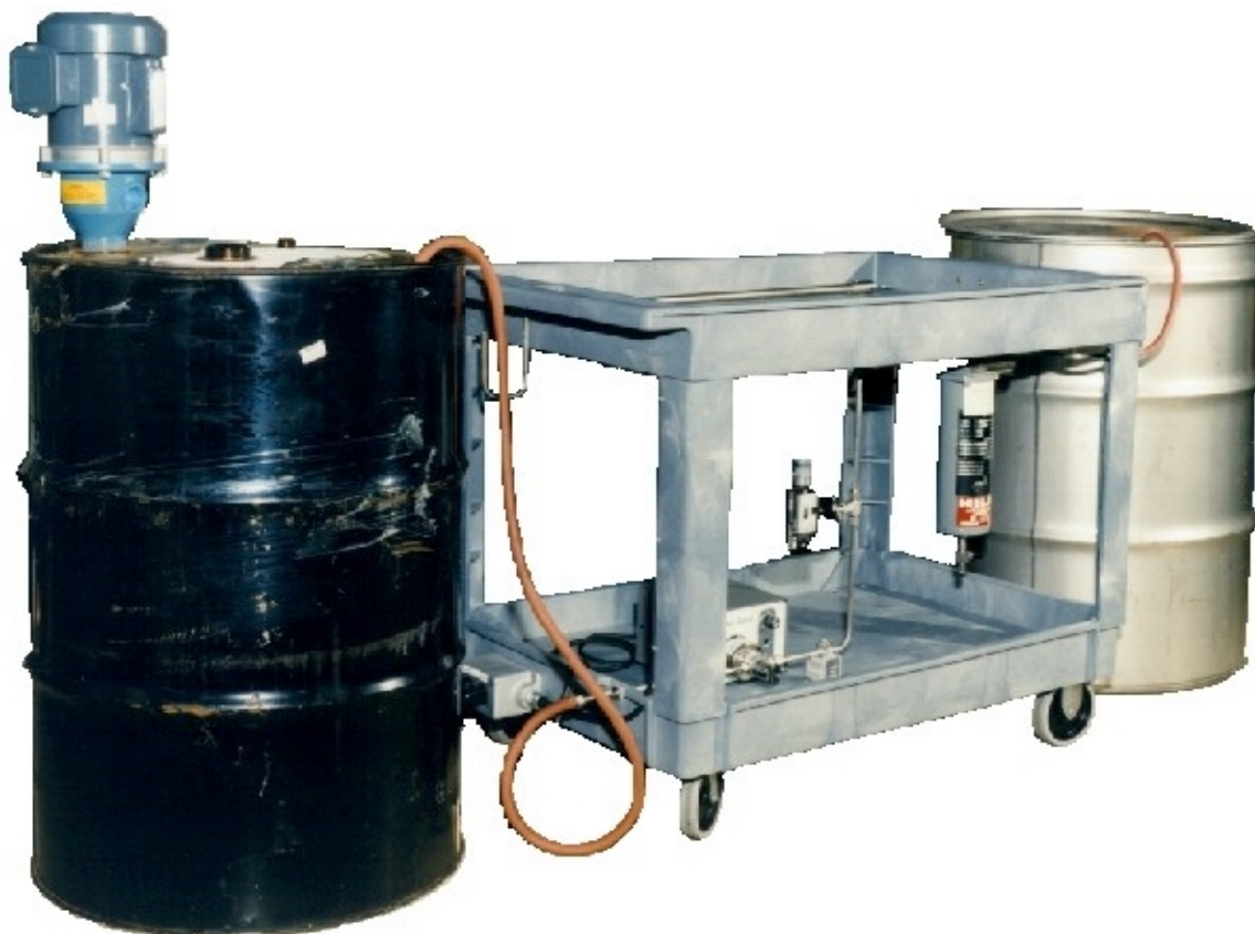
Fig. 4. Photograph of the mercury-in-oil removal process (MORP).
