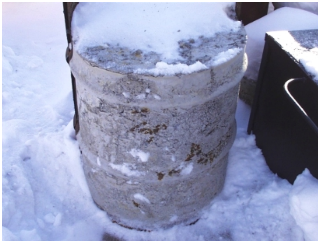
Fig. 2. The cut barrel with a cement compound sample, prepared by a method of impregnation with high penetrating cement mortar on the base of nonradioactive ash.
