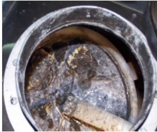
Fig. 4. The container with radioactive ashes from plant "Torch", treated by a method of impregnation with high penetrating cement mortar.
