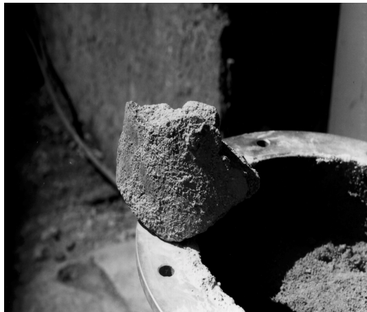
Fig. 1. Filter - patron with a ferrocyanide type sorbent, treated by high penetrating cement mortar, with a cement compound sample taken out.
