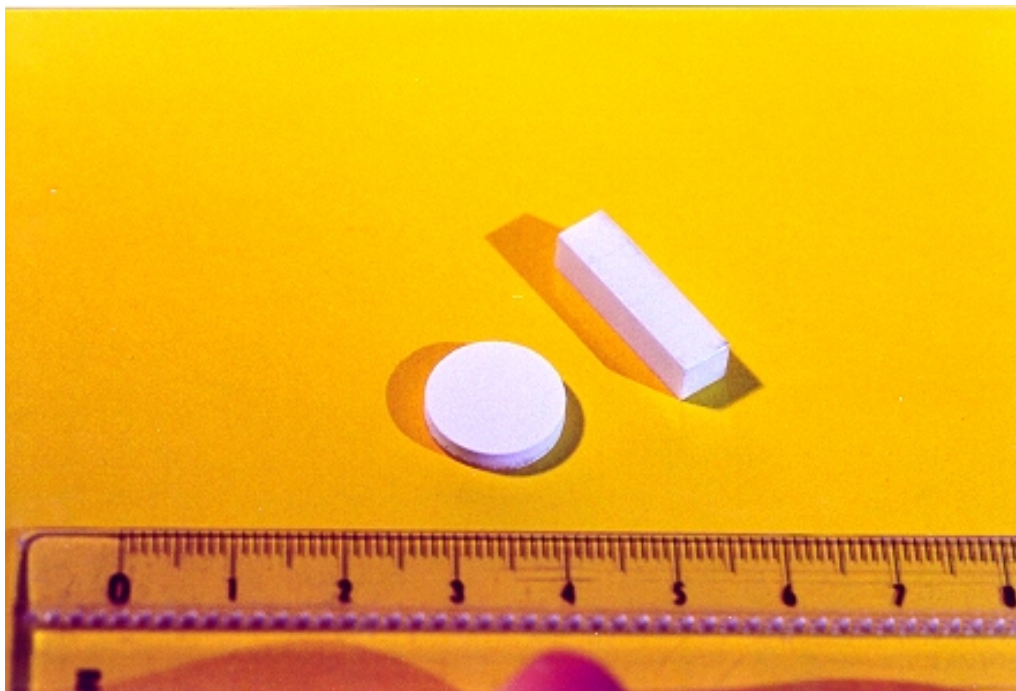
Figure 2. Sintered samples of TPD (the scale is given in centimeters).
