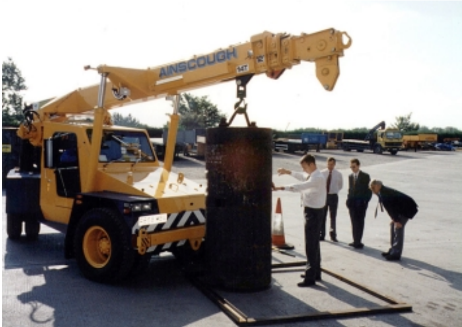
Fig. 3. Inactive Commissioning Trials of the Specialist Crane
