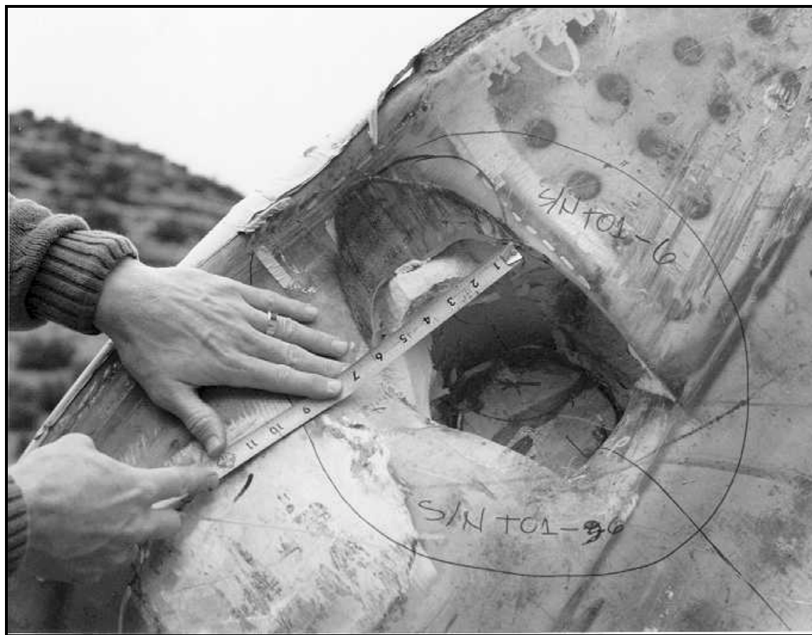
Figure 2 Puncture Damage to the TRUPACT-II Packaging Outboard of the Closure Regions
