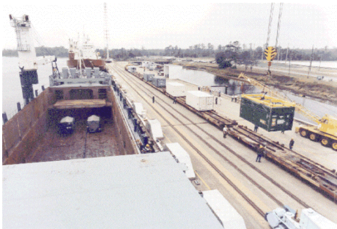
Figure 1 - FRR SNF Shipment Offloading Operations
