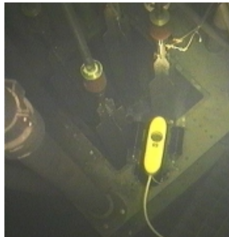
The RUCS vehicle inspecting a control rod on the ARMF reactor
