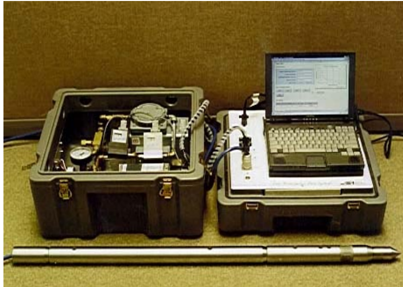
Fig. 2. Pump box, data-acquisition system, and permeameter rod.
