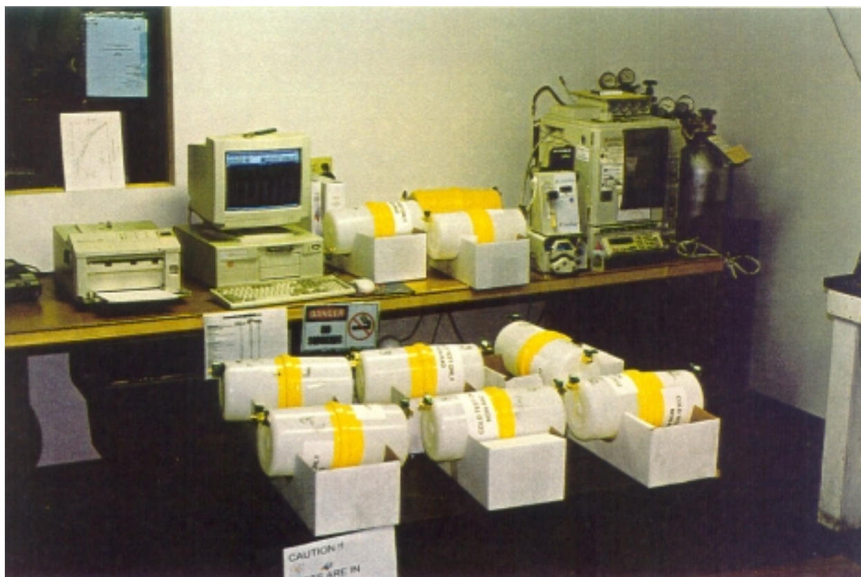
Photograph #1 - Shows the hydrogen gas test stand with the Gas Chromatograph, Computer, Peristaltic pump and several Clam Shells.
