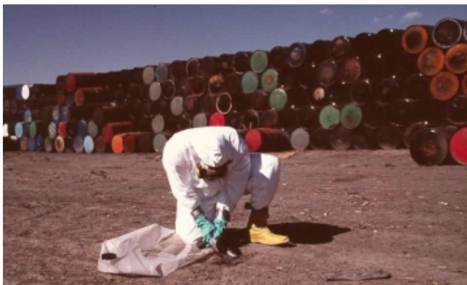
Fig. 1. Sampling Soil for Hazardous Waste While Facility Was Operational
