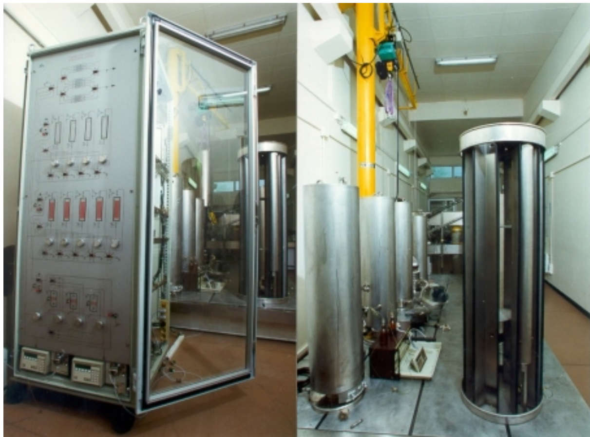
Figure 3 : photographs of the facilities : supervision system, tri-axial cells and supplying unit.
