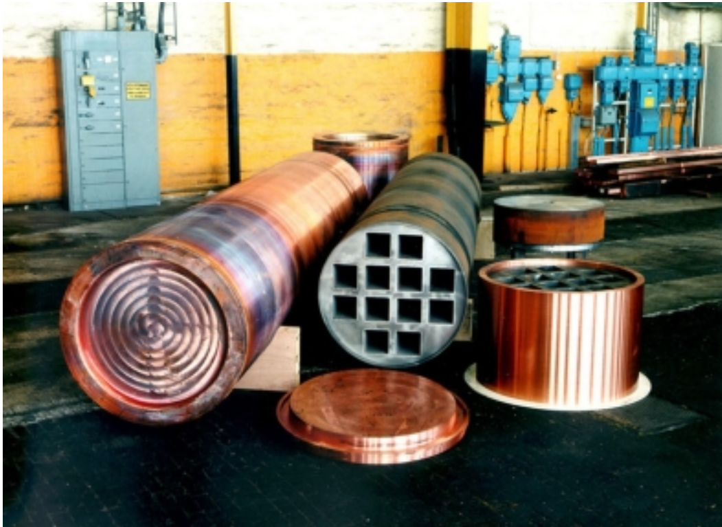
Figure 3. Copper canister with cast insert (reference design).
